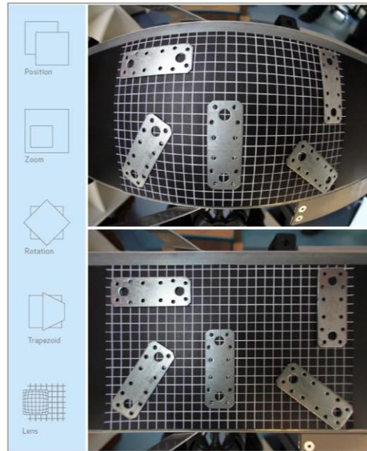
Fig.: Sample code - geometrical image correction in real-time with GigEPRO
