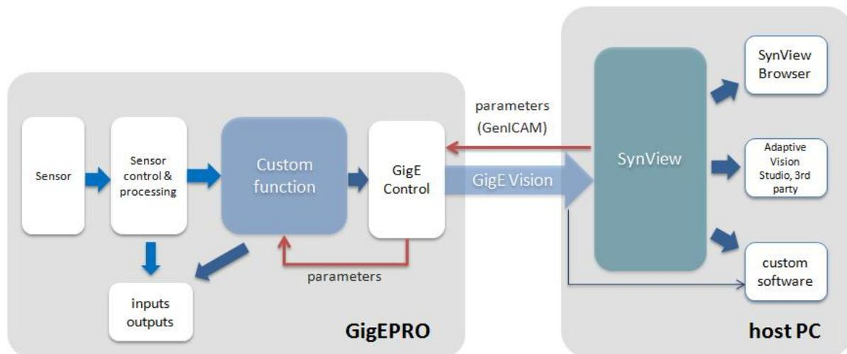
Fig.: Implementation of the Open Camera concept in the GenICam structure
