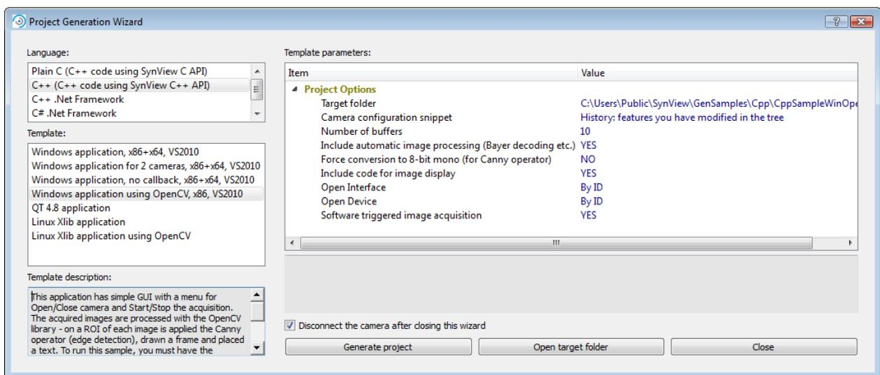
Figure 15: SynView Explorer: Source Code Generator configuration
