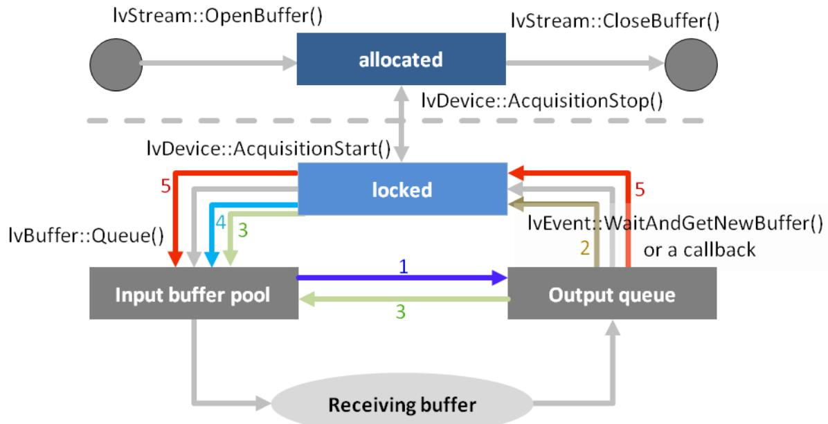
Figure 24: SynView: Flushing buffers
