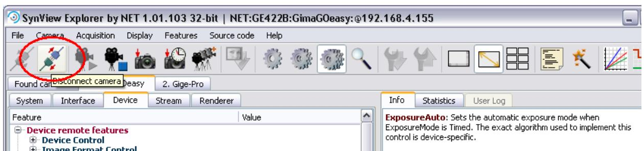
Figure 22: SynView Explorer: Disconnect the camera
