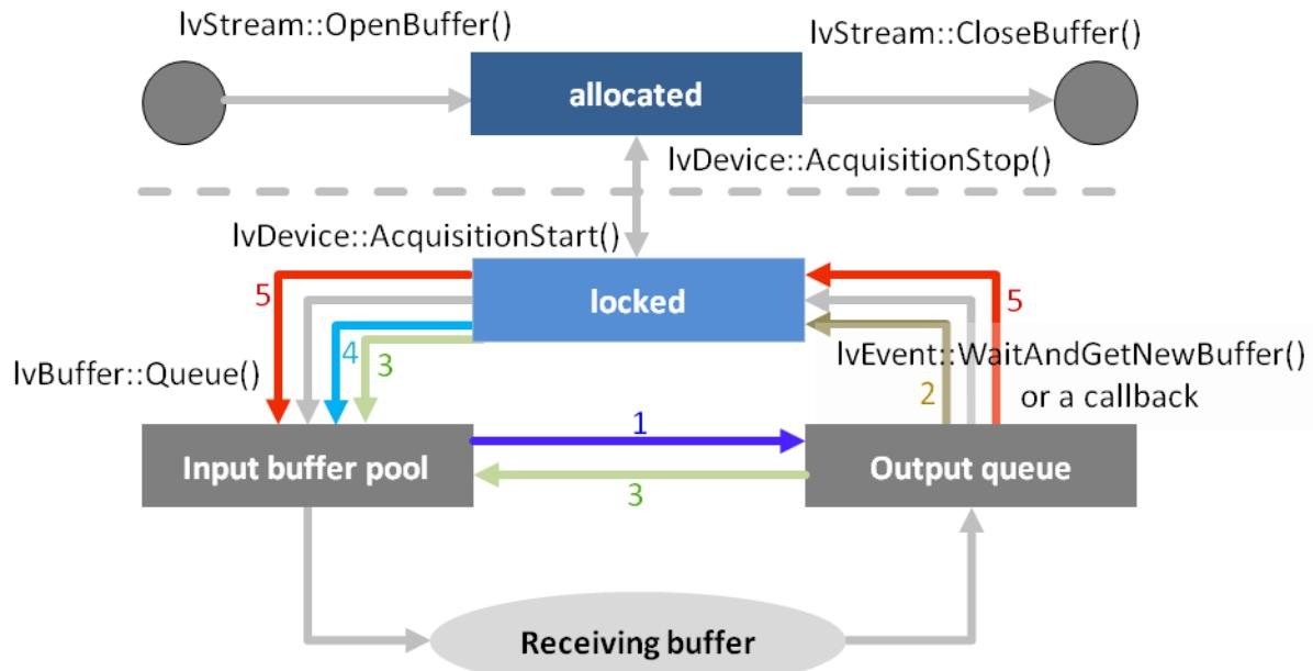
Figure 24: SynView: Flushing buffers
