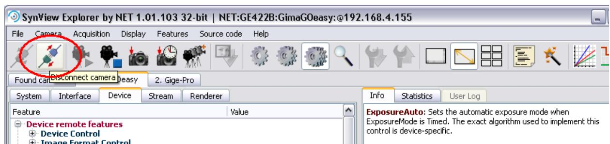
Figure 22: SynView Explorer: Disconnect the camera
