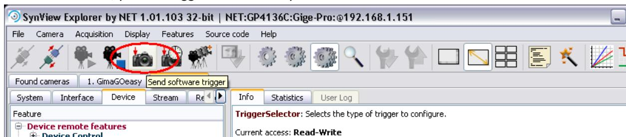
Figure 31: SynView Explorer: Trigger the camera
