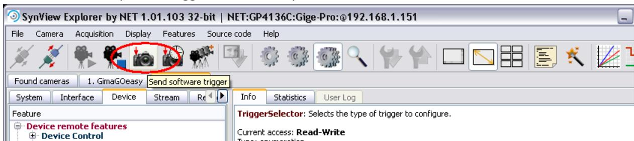
Figure 31: SynView Explorer: Trigger the camera
