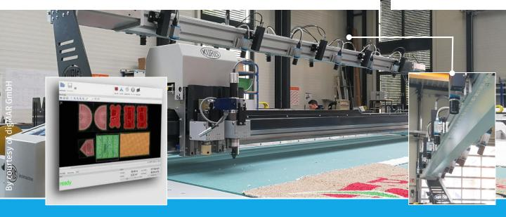
The Austrian company digMAR GmbH, a supplier of customer-specific system solutions, has decided to use NET's GigEPRO cameras with integrated real-time image processing for the carpet-cutting machines of its customer KURIS. NET's Open Camera Concept® allows customers to implement their own algorithms directly in the camera for unique vision solutions.
