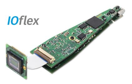
IOflex is an intra-oral camera solution for dental applications. With IOflex, videos and images are recorded and captured in full HD. The innovative feature enabling image enhancement directly in the camera's FPGA ensures excellent image reproduction and smooth video streaming. This means that even high-resolution videos can be transmitted to the computer via a USB 2.0 interface.
