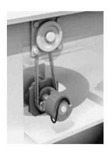
To simplify image processing, it is paramount to acquire images without any distortion, especially in line scan applications. An incremental encoder provides information about the current speed of the conveyor to the CORSIGHT smart vision system.
